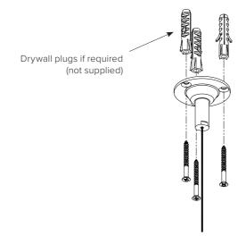
NOTE: when possible mount to studs or solid surface. Use drywall plugs only when necessary. Each cable gripper must be able to support 15kg.
