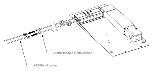
**Tunable White (TNW) Luminaires:** LED Panel cables plug directly into control module. Use control module outputs 1 and 3 for TNW luminaires.
