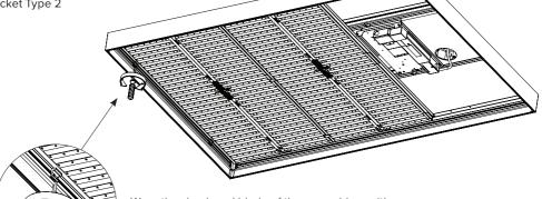
Wrap the shank and blade of the screwdriver with masking tape. Then remove panel support brackets by twisting the screwdriver carefully
