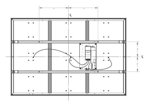
In the following charts, suspension points are taken from the geometric center of the frame.
